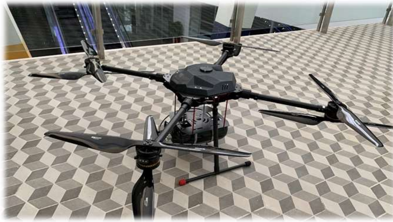
COAXIAL COPTER CUSTOMIZED DESIGN TO INCORPORATE FUEL CELL AS A PAYLOAD
