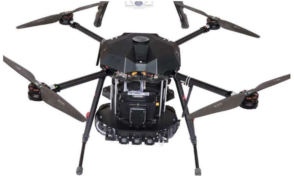
QUAD-COPTER WITH FUEL-CELL PAYLOAD
