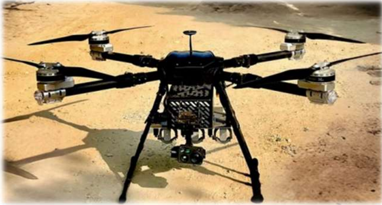
QUAD-COPTER WITH HAVING PALOAD RELEASING MECHANISM
