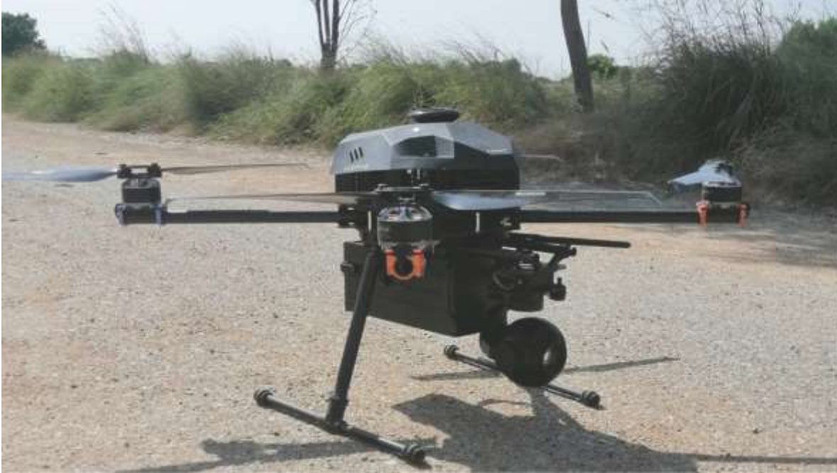
QUAD-COPTER WITH BATTERY COMPARTMENT AND GIMBAL
