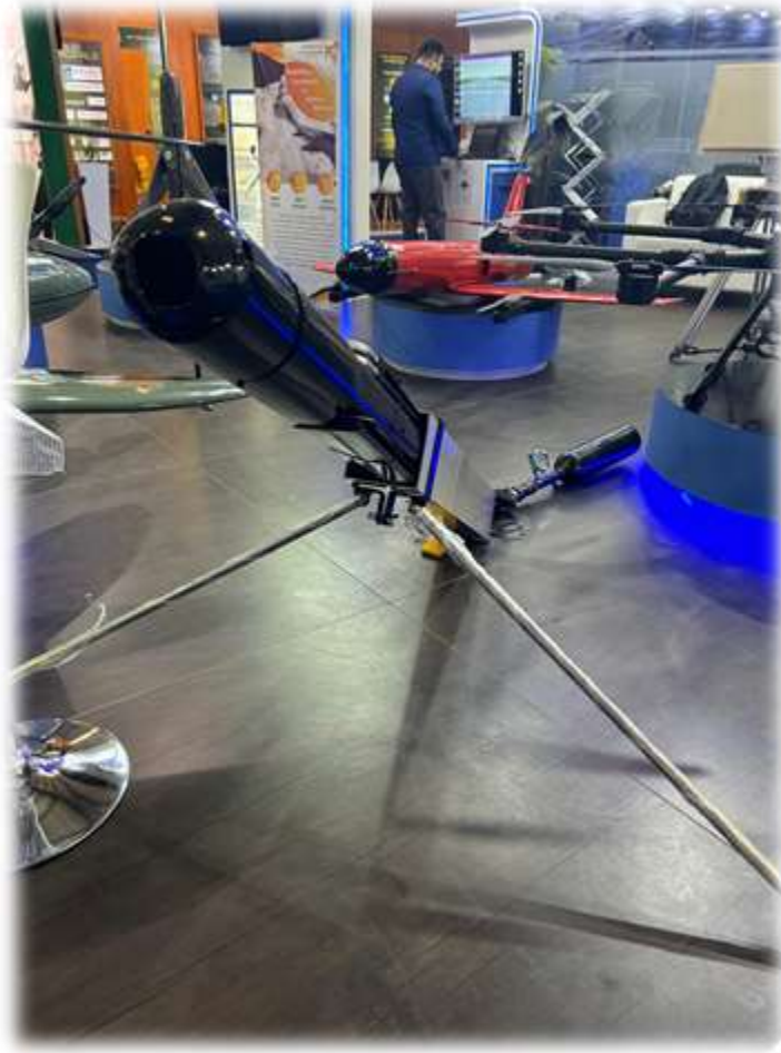
FOLDABLE LOITER MUNITION UAV IN PNEUMATIC TUBE LAUNCHER
